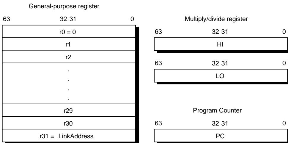
Figure 1-3. VR4111 CPU Registers
