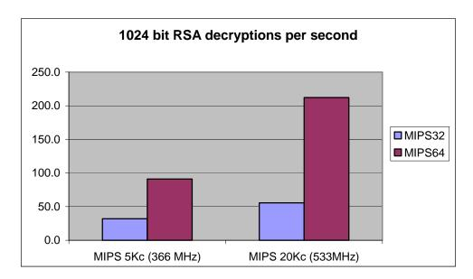
These estimates assume that the 5Kc and 20Kc processors are operating at 366 and 533 MHz, respectively, and that the RSA decryption package takes advantage of the Chinese Remainder Theorem. This theorem allows the 1,024-bit RSA decryption operation to be split into two 512-bit modular exponentiations, with some simple arithmetic to combine the results.
