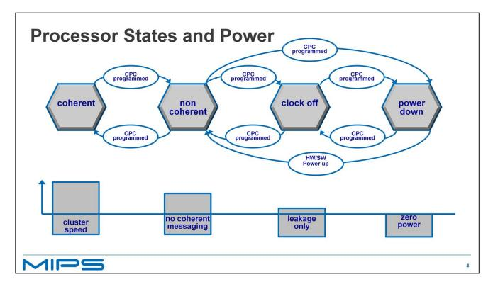
This slides shows the possible flow between Processor states along with some idea of power consumption.
