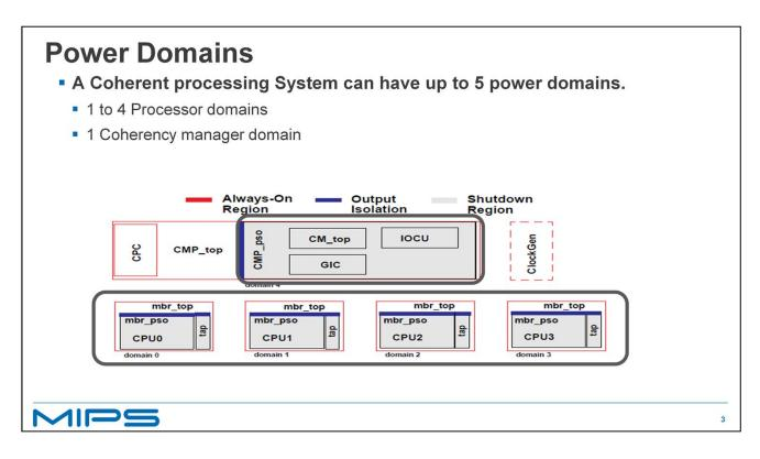
The cluster power controller breaks the coherent processing system down into isolated power domains. Domains that can shutdown are indicated in grey.
