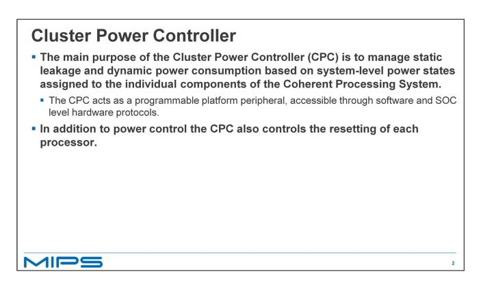
The Cluster Power Controller controls the power consumption in accordance with the system load. More processing elements can be powered up when needed and powered down when they are no longer needed.
