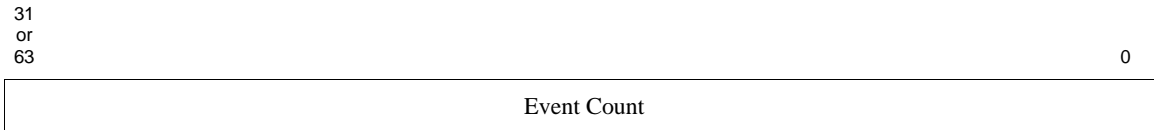
Figure 9.67 Performance Counter Counter Register Format
