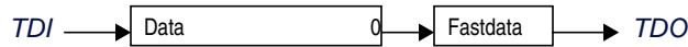
Figure 11.16 TDI to TDO Path When in Shift-DR State and FASTDATA Instruction is Selected
