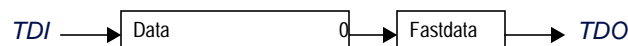
Figure 11.17 TDI to TDO Path When in Shift-DR State and FASTDATA Instruction is Selected
