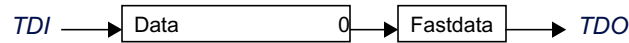
Figure 8.24 TDI to TDO Path When in Shift-DR State and FASTDATA Instruction is Selected
