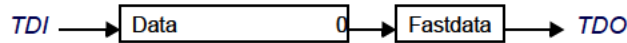
Figure 10.24 TDI to TDO Path When in Shift-DR State and FASTDATA Instruction is Selected
