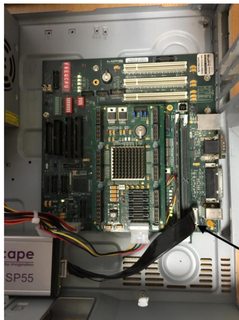
Figure 3 Connecting up a Malta + coreFPGA6 development board
