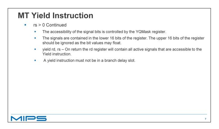
+ As I have previously covered in the MT control registers section the YQMask register enables particular Yield Qualifier pin signals so if the bit corresponding to the pin is not set a "invalid qualifier" exception will be generated and the OS can then decide what to do with the thread.
