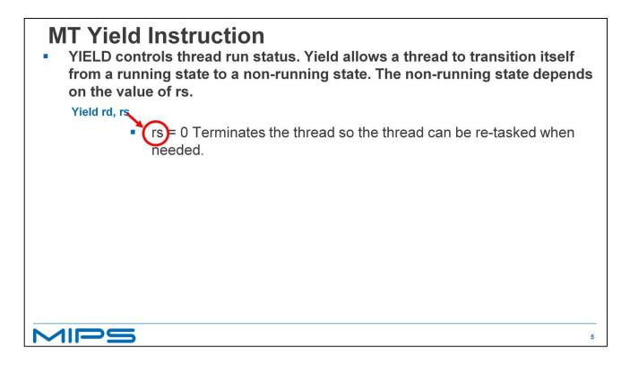
The Yield instruction allows a thread to control its execution. It can terminate itself, check for events to process or wait for events to happen.
