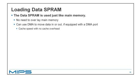
The Data SPRAM RAM block appears to your program as normal physical memory so there is nothing special you need to do once the Block is enabled.
