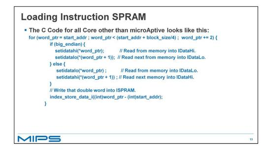
This code assumes you have already positioned the Instruction SPRAM directly over the code in main memory so that the starting address variable start\_addr is the starting address of the code to be copied in main memory and also the starting address of the Instruction SPRAM Block. The starting address is also assumed to be a kseg0 cacheable address. The block size is the size of the Instruction SPRAM block.
