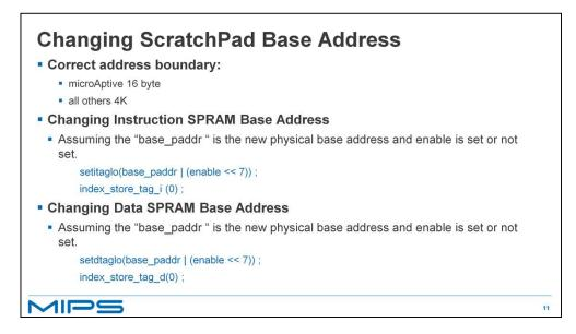
You don't need to stick with the default physical base address that was set at core build time. You can change it to anywhere in memory on correct boundary for your core
