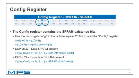
The CP0 Config register contains the SPRAM configuration bits
