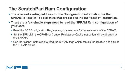
Configuration information for the ScratchPad blocks are keep in the SPRAM tag register.
