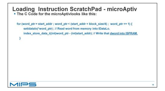
The code for the microAptiv cores it is simpler because there is no need to account for Endian because only 32 bits are written at a time.
