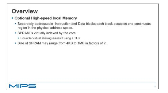
Most processor Cores support the option of adding high-speed local memory blocks during the building of the core. These blocks are referred to as ScratchPad RAM (or SPRAM). They provide low-latency storage for critical code or data. SPRAM access speed is similar to that of locked cache lines, but without impact on cache performance or maintenance.
