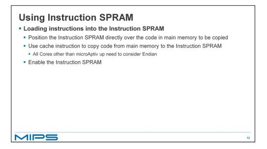
To get your code into the scratchpad, the instruction SPRAM block needs to be loaded from main memory using the cache instruction, index store Data.
