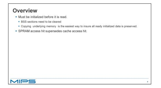
Software must ensure a SPRAM entry has been initialized the same as regular memory before it is read, to avoid reading spurious data.
