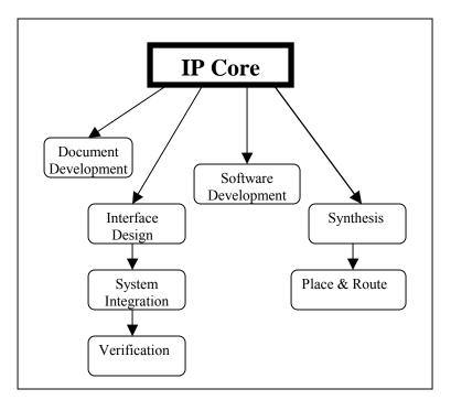
Figure 1: Development tasks affected by IP cores
