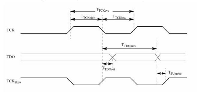
Figure 2 TDO Timing at Probe with Skewed Probe Sample Clock
