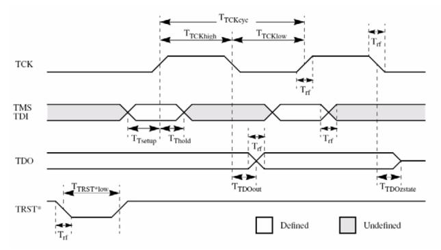
Figure 1 Test Access Port Signals Timing
