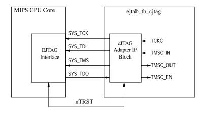
To see how the adapter works, TAP-related test cases such as 'tap\_fastdata-ebm32k-cjtag-zws' can be run under a normal softcore testbench environment. Without the '-cjtag-' mode string, the test cases will run with the normal EJTAG (IEEE1149.1) interface, bypassing the Adapter.
